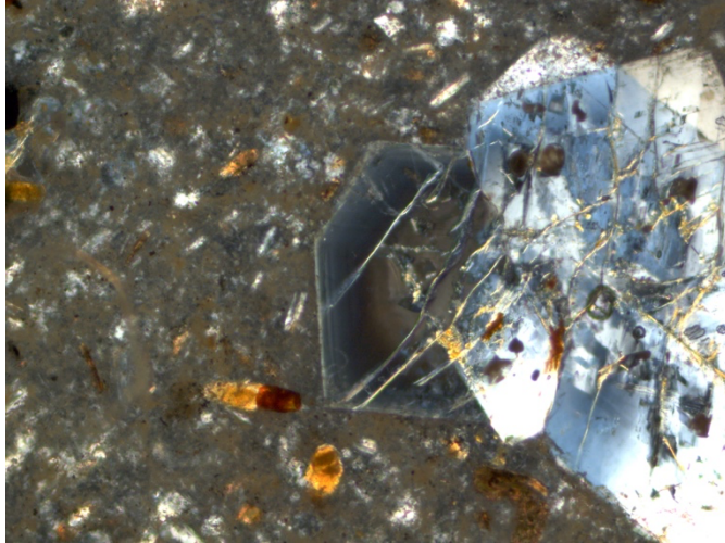
Figure 2. Upper left shows broken feldspar (PL, 10X WOF 1.1 mm). Upper right illustrates resorbed feldspar below plagioclase with euhedral termination. Brown minerals are hornblende. Lower left (20x, XP, WOF = 0.55 mm) shows euhedral feldspar, likely sanidine). Lower right (10X, XP, WOF = 1.1 mm) is a zoned but euhedral feldspar.
