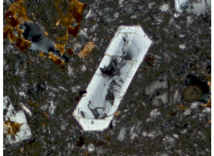
Figure 2. Upper left shows broken feldspar (PL, 10X WOF 1.1 mm). Upper right illustrates resorbed feldspar below plagioclase with euhedral termination. Brown minerals are hornblende. Lower left (20x, XP, WOF = 0.55 mm) shows euhedral feldspar, likely sanidine). Lower right (10X, XP, WOF = 1.1 mm) is a zoned but euhedral feldspar.
